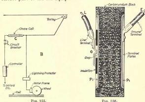
Fig. 155.—Protector on car, alternative arrangement.
